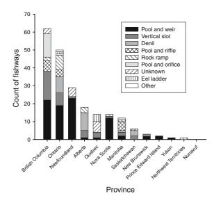
Fig. 2 Count of fishways by province or territory. Conventional-type fishways are displayed in *gray scale* and nature like fishways are displayed with *crosshatching*. Eel ladders were displayed with *vertical crosshatching* to differentiate them from conventional type fishways. One fishway is listed as in the "other" category, this fishway is unique in its design and does not fit into the other categories
