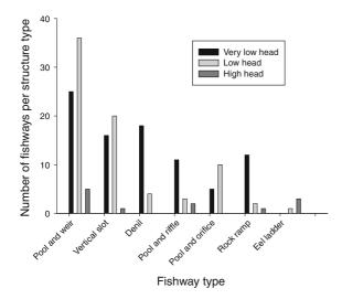
Fig. 3 Number of fishways per dam category for the different types of fishways contained in the CanFishPass database. Dams were separated into three categories; the very low head category contained dams <3 m in head-height, the low head category contained dams equal to and >3 m but <10 m in head-height, and the high head category contained dams equal to and >10 m in head-height. Head-height data were available for 175 of 212 fishways
