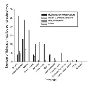
**Fig. 6** Number of fishways per structure type for each province. The hydropower infrastructure grouping represents fishways that were installed to mitigate the effects of both hydropower dams (n = 28) and natural barriers (n = 11) exposed by hydropower operations. The 'other' grouping consists of hatchery fences, all of which are in British Columbia (n = 7), and lamprey barriers (n = 5) which are all located in Ontario
