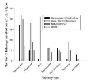
**Fig. 4** The number of fishways by barrier type is shown for different fishway designs. The hydropower infrastructure grouping represents fishways that were installed to mitigate the effects of both hydropower dams (n = 28) and natural barriers (n = 11) exposed by hydropower operations. The other grouping consisted of hatchery fences (n = 7) and sea lamprey (*Pertomyzon marinus*) barriers (n = 5)
