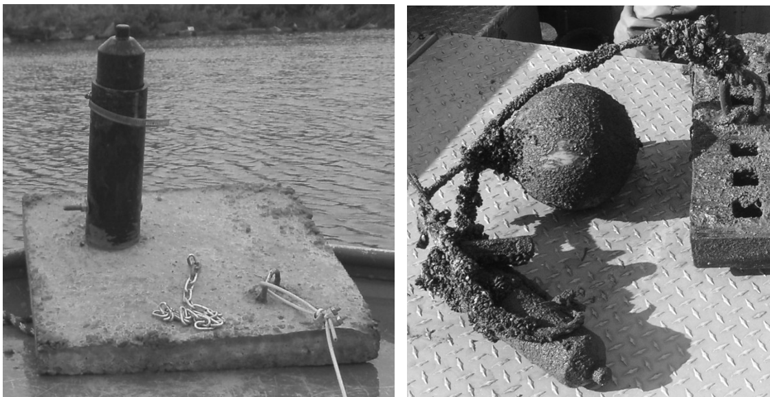
Figure 2-2 a) Custom-built cement station with embedded polyvinyl chloride PVC pipe and b) station covered with biofouling.
