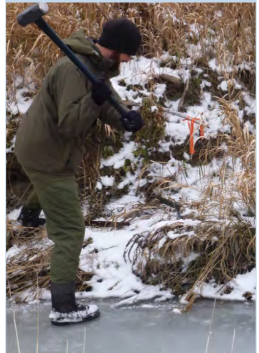
Installing erosion pins in Watts Creek
