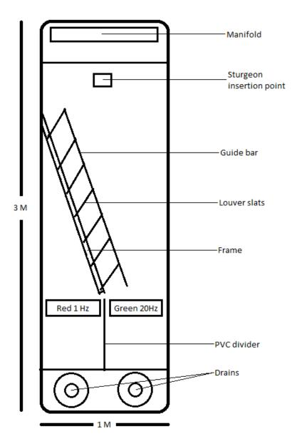
**Figure 3-1.** Schematic diagram of the raceway used to test the effectiveness of the integrated light-louver array on downstream passage of juvenile white sturgeon (*Acipenser transmontanus*). Louver slats could be removed entirely or spaced at 5 cm, 10 cm, or 20 cm. Distance between the LGD and the sturgeon insertion point is 200 cm.
