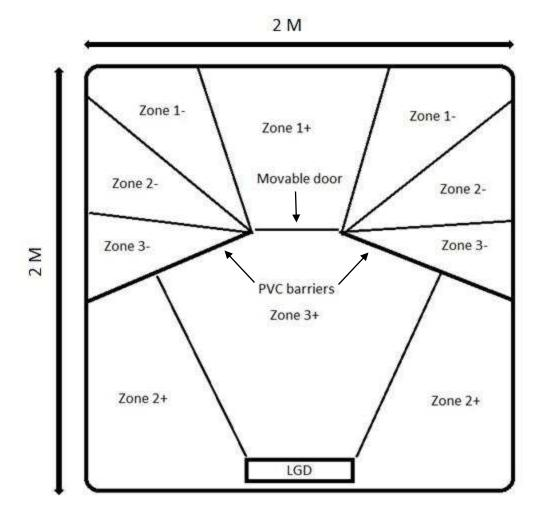
**Figure 4-1**. Tank setup with physical design and showing zone overlay used for analysis.
