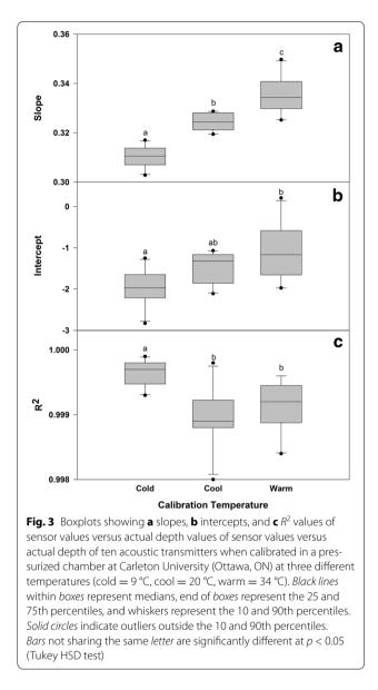
water, the equation reports depths of 67.88 and 68.41 m, respectively, instead of the actual depths of 68 m. Therefore, when using room-temperature pressures instead of pressures at the desired temperatures to calculate depths, transmitters at depths of 68 m in 4 or 40 °C fresh water can be reported 0.12 m shallower or 0.41 m deeper, respectively, than their actual depths (Table 1). This represents a maximum error of 0.006 m for each meter of depth.
