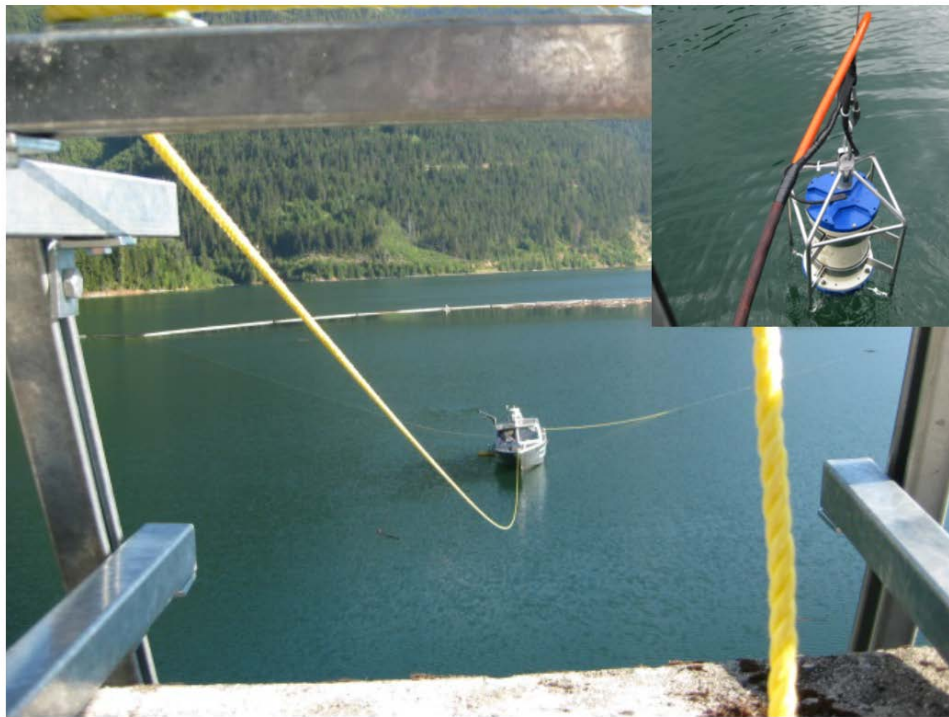
Figure 6: 3-point mooring system used to secure the boat during flow and temperature sampling in the forebay of Mica Dam. The inset image shows the ADCP unit used to collect flow and temperature data.
