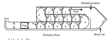
Fig. 1. Schematic of the Vianney-Legendre vertical slot fishway on the Richelieu River in Quebec, Canada. Numbers 1–5 indicate fishway sections and corresponding basins. Distance metrics, corresponding to locations of PIT antennas, indicate the cumulative minimum transit distance between successive fishway basins (beginning at 0 m) and were used in calculations of distance moved and location.
