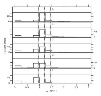
Fig. 3. Frequency distribution of lake sturgeon (n=30) swimming speeds ( $U_{\rm s}$ ; m s<sup>-1</sup>) through pooled basins located in different sections (1–5) of a vertical slot fishway. The black dashed line indicates the critical swimming speed ( $U_{\rm crit}$ ) of the average sized sturgeon in this study, and grey dashed lines indicate minimum and maximum  $U_{\rm crit}$  values for the smallest and largest individuals, respectively.
