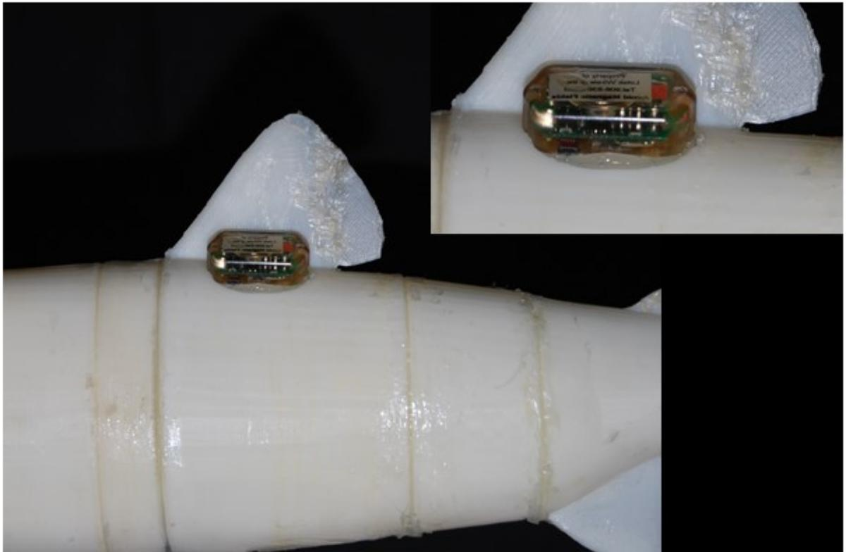
**Figure 2.2:** Photograph of the model with an attached electronic tag to illustrate placement and method of attachment. Inset is an enlarged view of the tag at the base of the dorsal fin.
