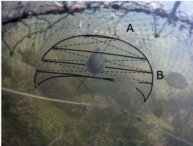
**Figure 6.** The escape opening (A) and selective grid (B) of the prototype passive in-net turtle escape device (PIN-TED) used in field trials in Lake Opinicon, Ontario, Canada, in July 2012. An adult painted turtle *Chrysemys picta* is passing through the selective grid. The grid has been traced with black lines while tarred twine has been traced with dashed lines.
