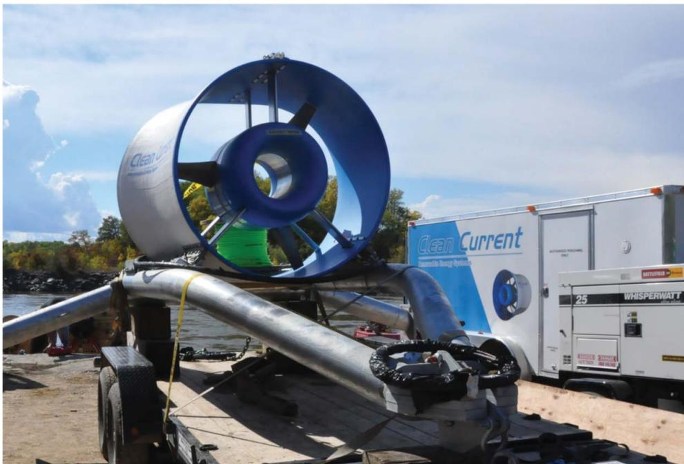
**Figure 3.** Ducted axial-flow hydrokinetic turbine that was installed and being testing by Clean Current Power Systems (Vancouver, BC) at the Canadian Hydrokinetic Turbine Testing Centre on the Winnipeg River, MB, Canada.
