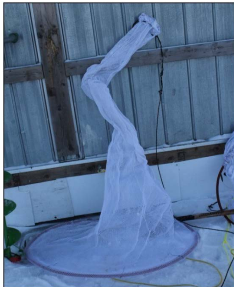
Picture 3. A photograph of the sub-surface holding pen for Walleye. The net presented here was recently removed from the lake and was frozen from cold air temperatures. The pen had approximate dimensions of 0.5 m radius, 1.9 m height, for a volume of 0.5 m 3 .
