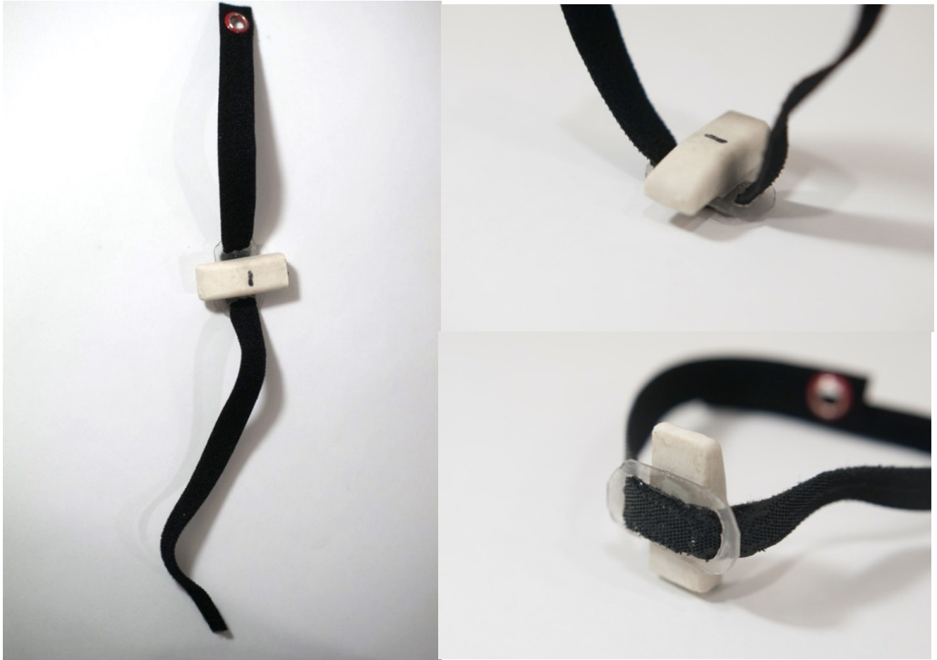
Figure 2.1. A Velcro® harness (black) and the biollogger (white). The biollogger was secured to a small plexiglass plate using marine epoxy and the Velcro® was threaded through small slits on each end of the plate.
