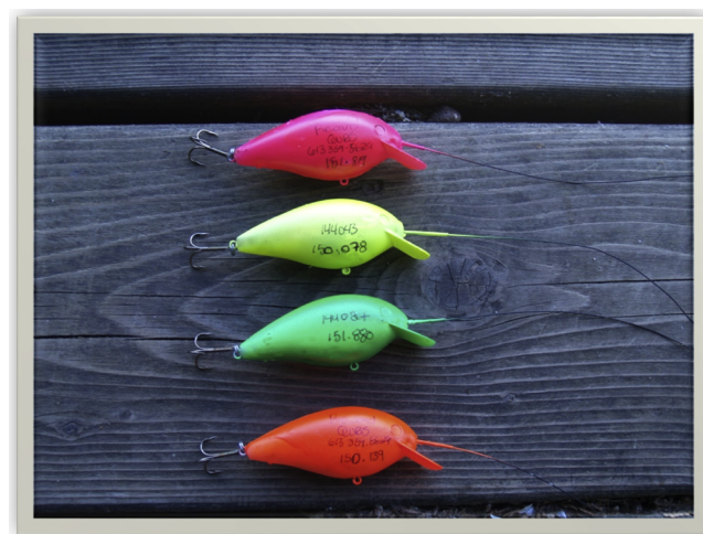
Fig. 1. Lure treatments included one treble hook at the posterior end of the lure assembly. The transmitter was embedded inside the lure body with the antenna extending out the anterior of the lure. Each colour was assigned to a specific treatment group for ease of recognition once assigned to a fish as well as for locating at a distance on the surface of the lake. Each lure was labelled with transmitter information, research affiliation and contact number. A nominal reward was provided to individuals who returned found lures. (For interpretation of the references to colour in this figure legend, the reader is referred to the web version of this article.)
