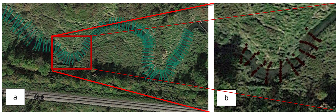
Fig. 2 Total station bathymetric points collected during summer: (a) 2014 (b) 2016. Flow from left to right. Background pictures taken from Google Earth
