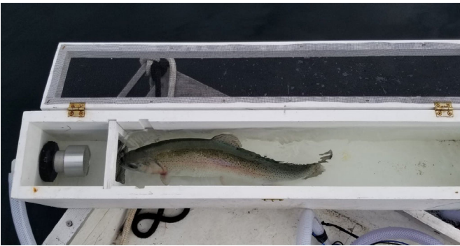
FIGURE 1. Rainbow Trout held in the flow box. Fish were positioned facing the direction of the flow, and the lid was closed during the treatment.
