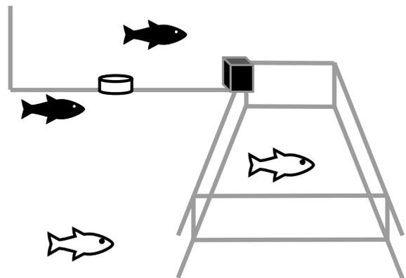
**Fig. 2** Schematic drawing of the BRUVS stand with camera position and bait arm. The camera stand and bait arm are represented by the gray lines, the camera (black cube) faces left towards the bait container, represented by the white cylinder. The solid black fish show how fish attracted close to the bait container will be recorded while the black outlined fish show how species which relate strongly to the substrate or structure would be less likely to be seen
