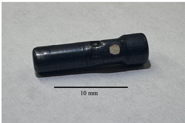
**FIGURE 1** V3D predation tag with an intact biopolymer coating (white). This predation tag weighs 0.33 g in air, has a 141-dB acoustic power output at 307 kHz, and has dimensions of 4.0 mm diameter × 15.5 mm length.
