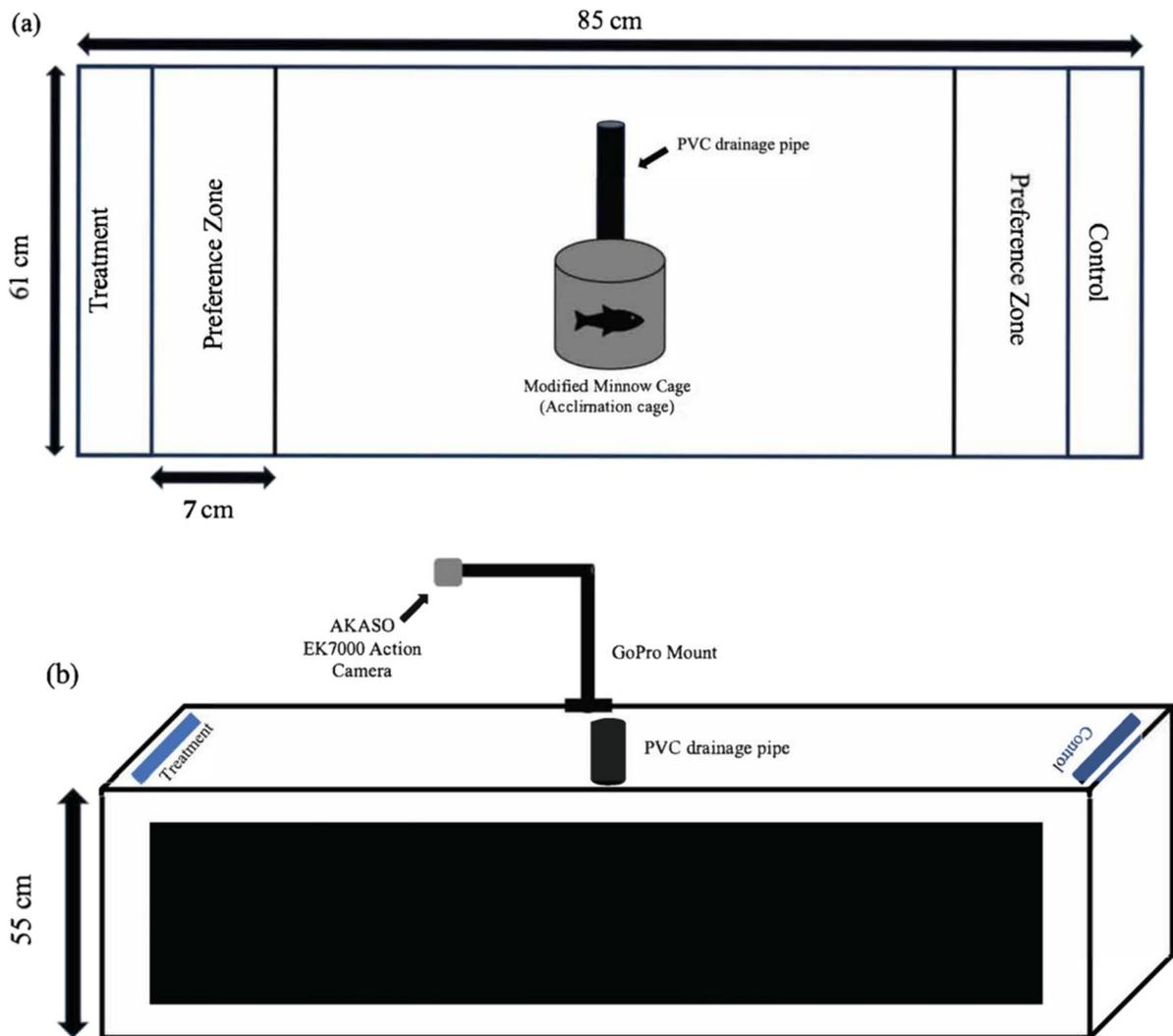
**Fig. 1** Experimental setup for investigating bluegill preferences in a fiberglass raceway trial arena. **a** The trial arena, measuring 85 cm in length, 61 cm in width, and 55 cm in depth, featured retaining walls with different textures and structures at either end. **b** Cameras were strategically mounted using a C-clamp affixed to two poles (122 cm base and 45 cm
