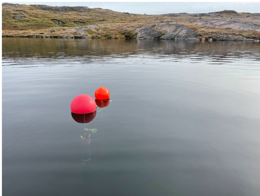
Figure 7: These buoys and sondes (EXO2) are deployed for weeks at a time to measure high-frequency changes in oxygen, temperature, conductivity, algal biomass, and fluorescent dissolved organic matter. The aim is to quantify lake metabolism. One of the constraints on such ecosystem monitoring is the need to replace the batteries and service the sensors every few months, making long-term deployments (e.g. over winter) difficult. Photo by Blake Matthews taken on a lake in Qassiarsuk, Greenland, September 2021.
