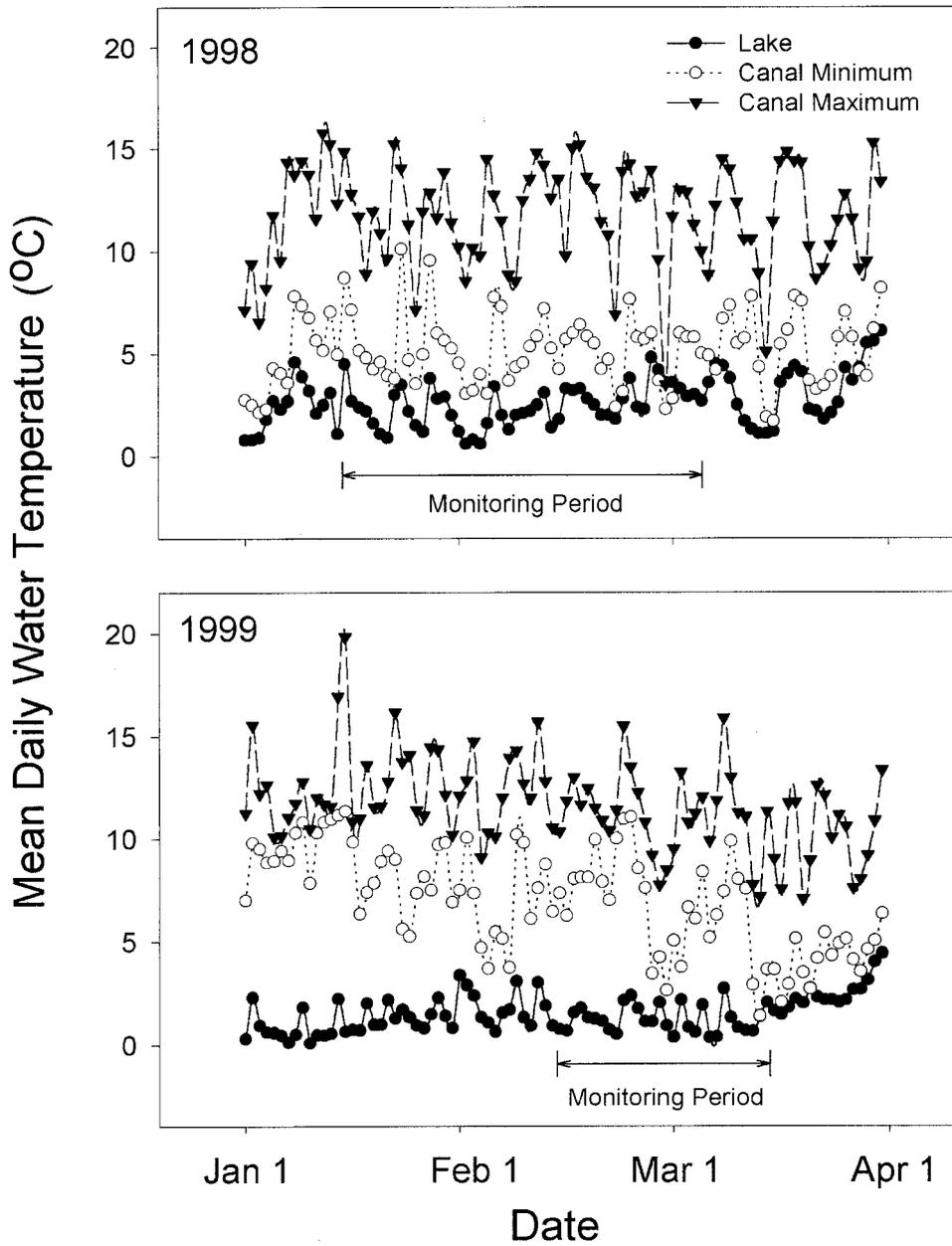
Figure 2. Thermal profile of water in the discharge canal and adjacent Lake Erie. Water temperatures are plotted for 1 January until 31 March in both 1998 and 1999. The lake temperature is based upon a daily mean calculated from half hour temperature records. The canal temperatures are based upon the daily maximum hourly temperature and the daily minimum hourly temperature. The periods during which fish were monitored in each year are indicated on the figures.
