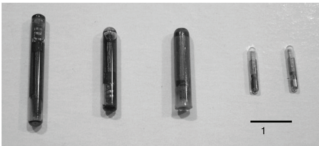
Figure 18.2 Passive integrated transponder (PIT) tags. The three larger tags on the left are half-duplex (HDX) tags, and the two smaller tags are full duplex (FDX) (photo by S. Cooke).
