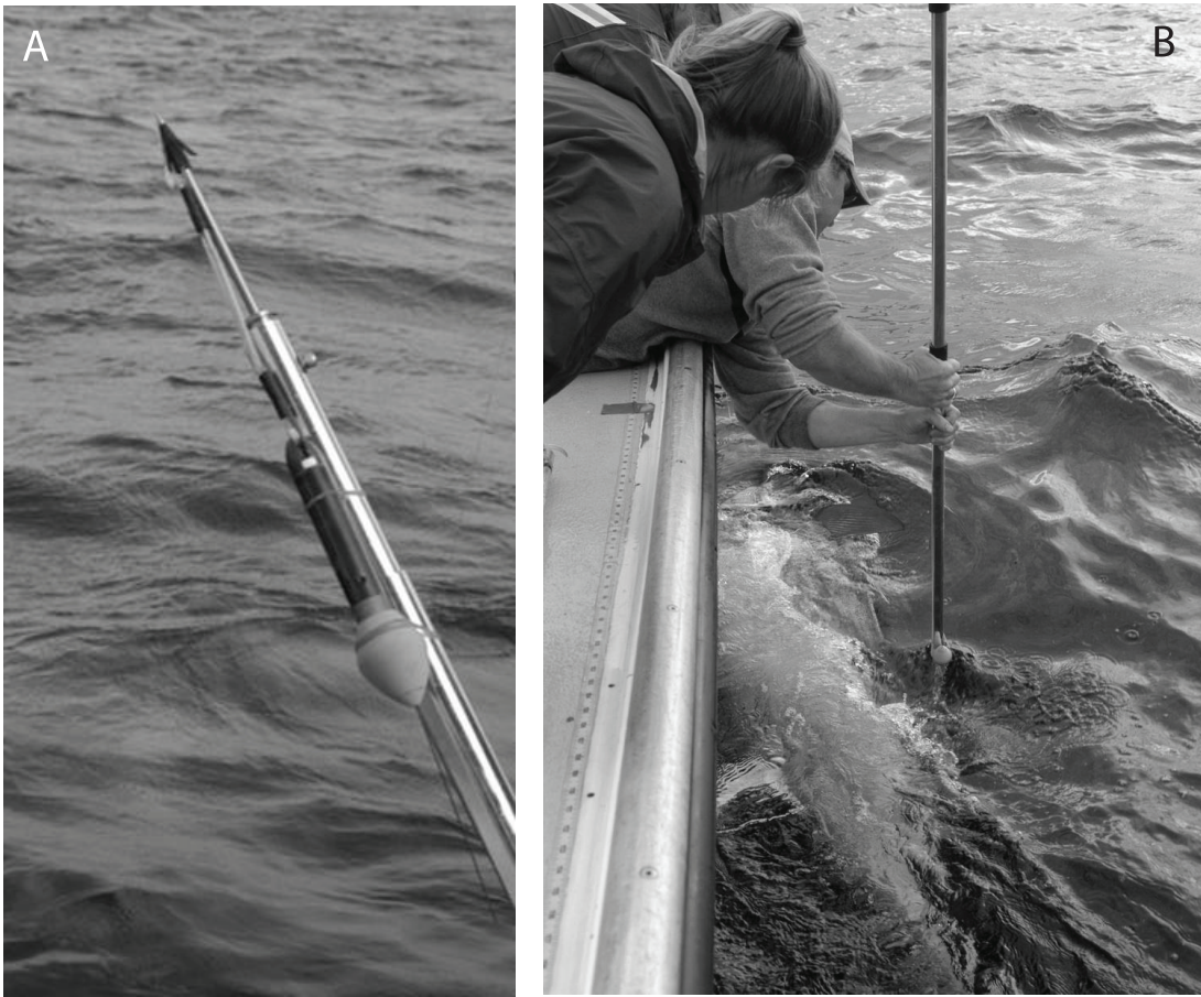
Figure 18.1 (A) Pop-up satellite archival tag (PSAT) attached to dart and mounted on a tagging pole; (B) dart being plunged into the dorsal musculature of an Atlantic bluefin tuna alongside tagging vessel (photo [A] by A. Speers, Dalhousie University, with permission; photo [B] by M. Stokesbury, Acadia University, with permission).
