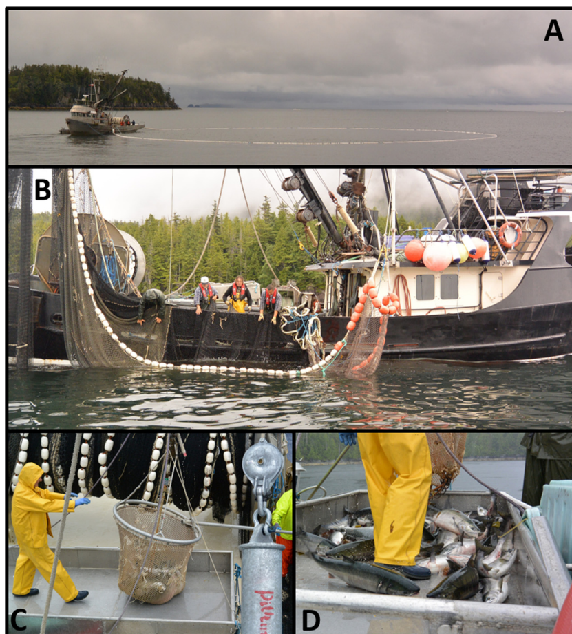
Fig. 2. Experimental capture was conducted from commercial purse seine vessels and simulated standard operations. Following deployment of the seine (A), the net was brought aboard with a drum until just the bag of the net was ‘pursed’ alongside the boat (B). Fish were held in the pursed net for a pre-determined amount of time and then transferred to a sorting table on deck using a brailer (i.e. a large dip-net; C) and sorted according to treatment (D).
