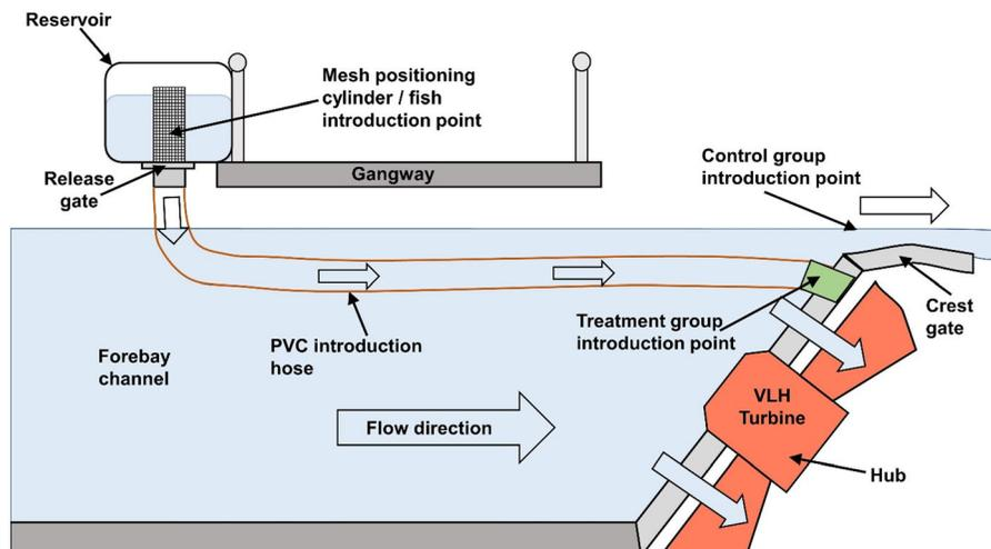
**Fig. 1** Schematic of the experimental entrainment apparatus used to experimentally entrain fish through the VLH turbines at Wasdell Falls, on the Severn River in Canada. The fish rested within the mesh positioning cylinder within the filled stock tank.
