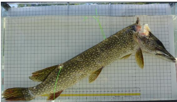
**Fig. 2** The single direct mortality observed in this study of the effects of entrainment on fishes through the VLH turbines at Wasdell Falls on the Severn River, Canada. This northern pike experienced a catastrophic partial decapitation
