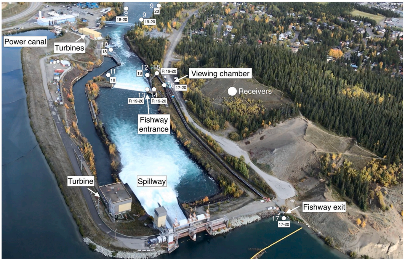
Fig. 2. Map of the hydroelectric facilities in Whitehorse, YT, and receiver locations from 2017 to 2020. All receivers were acoustic aside from those with a subscript 'R' which were radio telemetry receivers. Subscript numbers indicate the years that receivers were deployed at that location.
