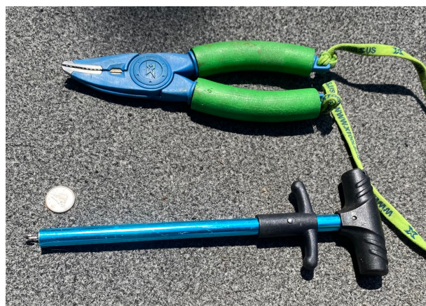
Figure 1. Hook removal devices used in this study: T-shaped mechanical dehooker (bottom) and needle-nose pliers (top), with a dime (Canadian 10-cent coin) for scale.
